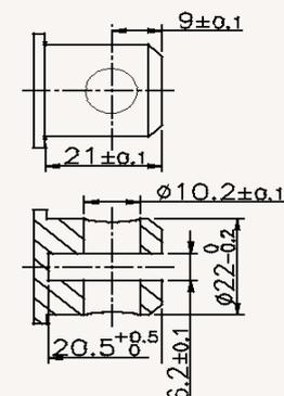
2=clevis head, width 6.2, depth 20, hole dia 8.2MM
