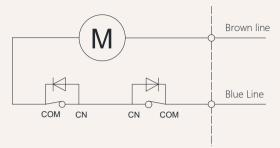
Schematic diagram of the internal circuit of the Hall signal
