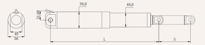
S: Stroke L: Retracted length L= Stroke +320mm >=400MM, L= Stroke +350MM
