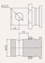
M1= Type M, M16 thread, depth 25 mm
