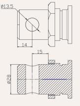
M2= Type M, M18 thread, depth 25 mm
