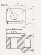
U1 = U-shaped, groove width 10.5mm, hole diameter 12.5mm
